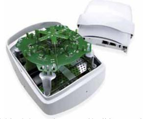
Patented smart antenna arrays in every access point provide longer range and more reliable Wi-Fi connections, requiring fewer APs than competitive alternatives.
